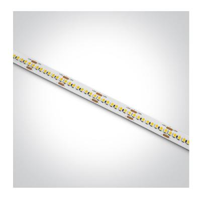
Flexible LED light strip, with SMD2835 LEDs, 240LEDs/meter, 42W/meter.Supplied in 5 meters roll with white PCB and double adhesive tape for a better fixing.
